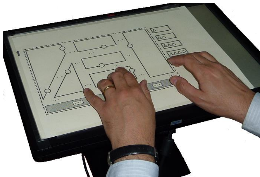
Figure 3: Interactive audio-tactile map prototype composed of a multi-touch screen with raised-line overlay
